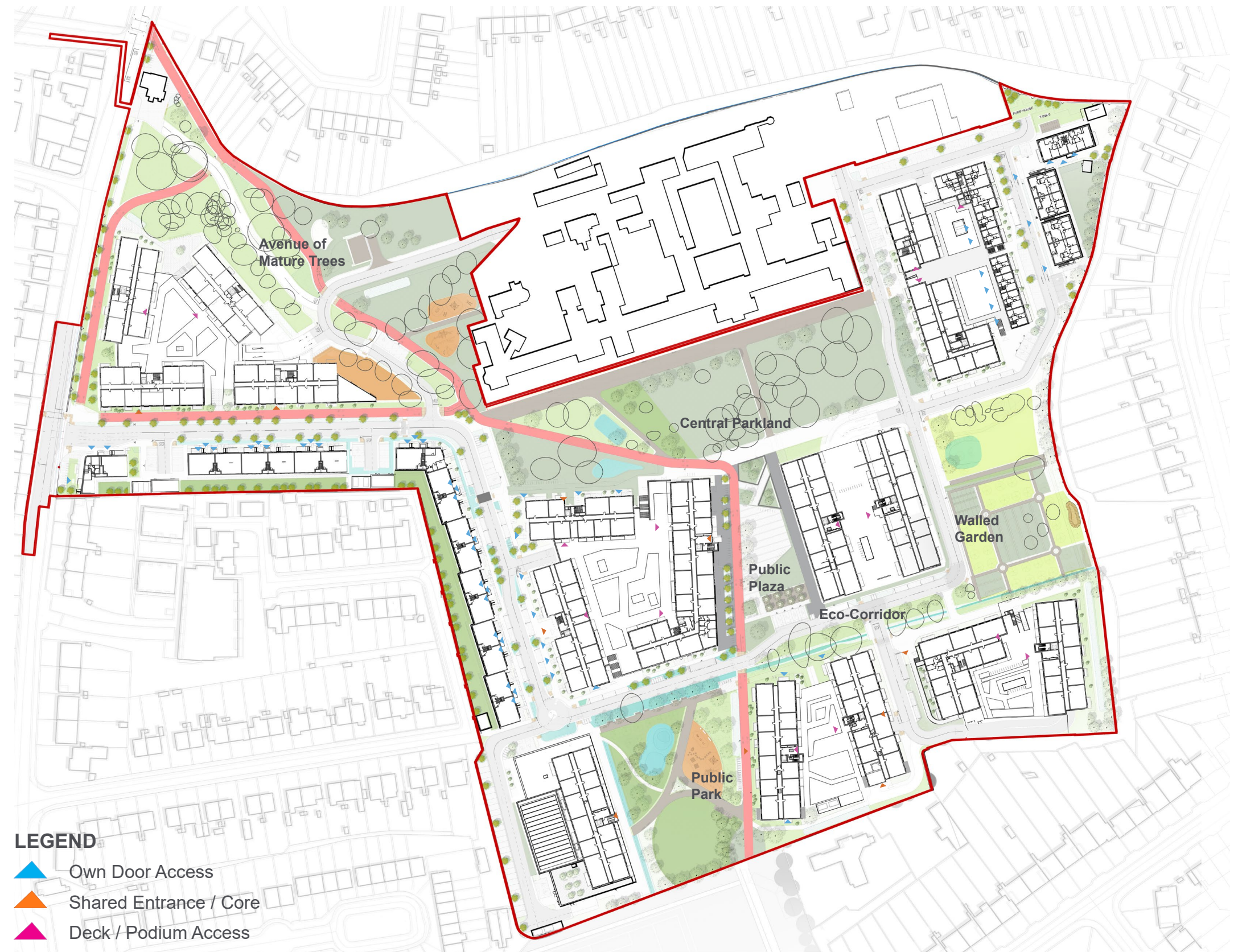
Figure 9 - Ground Floor Plan showing access to blocks (yellow) and own-door units (blue)
